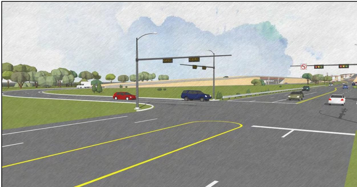
Figure 9. Build Alternative: Artist rendering (street-level view) proposed button-hook exit ramp at RM 620 and Deerbrook Trail
